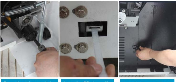
Press the stripper switch with left hand Insert the PP strap with your right hand
