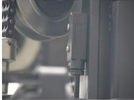
Lifting limitation function. When the forks are raised to the maximum height, the system will automatically cut off the power supply for lifting, and smoothly stop. This action not only can save energy, and prevent danger, but also extend the service life of the hydraulic systems and related components.
