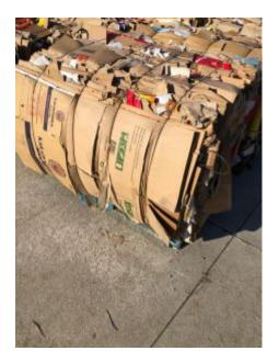
The clamping force of hydraulic hoses is used to compress the waste material. The bonded material is compressed to reduce the volume of the waste material. The baling procedure is as follows:
